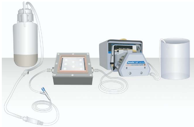
Figure 1. Diagram of the continuous flow system.
