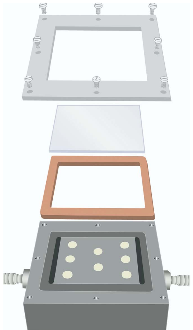
Figure 2. Diagram of the flow cell used to generate the biofilms.
